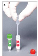
Insert pipette tip into the clear liquid in the control vial.
